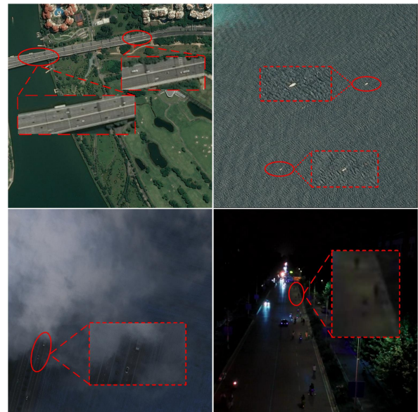
Figure 1: A demonstration of characteristics of small objects. The images in the first row depict small objects with a significant absence of critical information, while the images in the second row illustrate the vulnerability of these small objects to interference from environmental noise.
